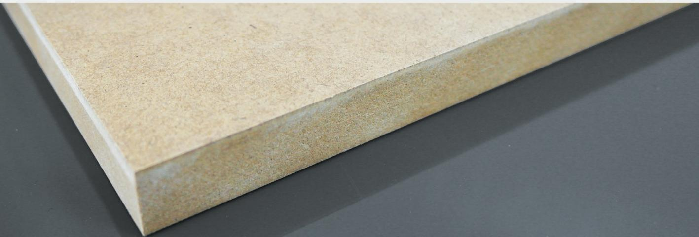
MDF, also called medium-density fiberboard, is made of pressed conifer wood fibers, and is used in the furniture sector for carcasses, drawers and fronts. Moreover, MDF is also used as base material for desks or cabinet systems. Because of the high bending- and tensile-strength and the smooth surface, the fiberboard is very popular.
