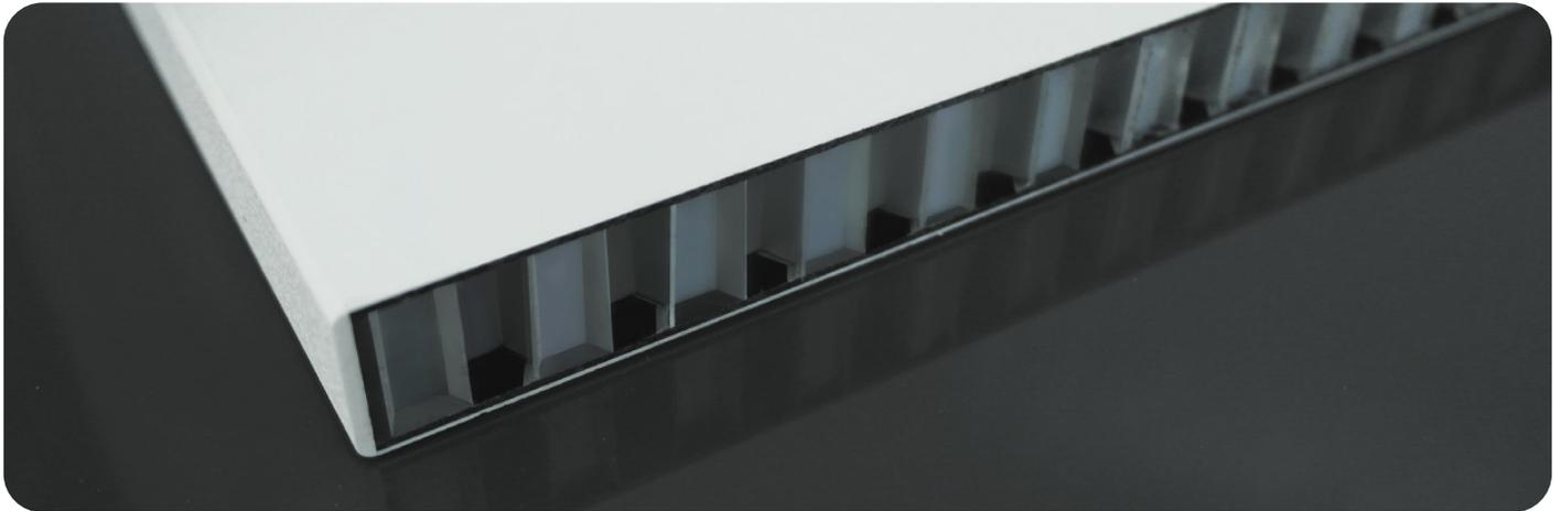
The honeycomb panel is made of a three-layer-construction with sandwich-structure, consisting of two outer layer providing strength in tension and the inner honeycomb material. The special construction of these panels ensures a high mechanical stiffness with low weight. For this reason honeycomb panels are widely used for furniture featured in the aircraft-, boatbuilding- and caravan-sector.
